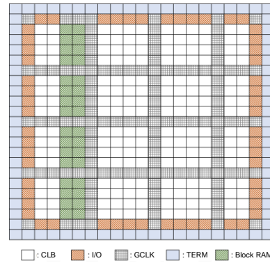
Fig. 3. Internal structure of the xc3s50 devices.
